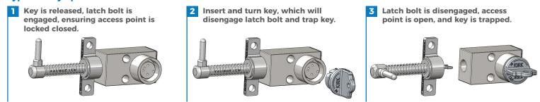
For HD multiple cylinder interlocks, all missing keys must be inserted and turned before any trapped keys can be released.
