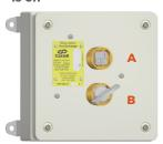
When the machine is running, key A is trapped in the key switch controlling the power. Key B is trapped in the mechanical time delay unit. This key is used to access the machine area, once machine has stopped running.
