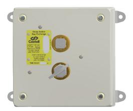
The DAE is a key controlled mechanical time delay unit designed to control access to dangerous machines which have a run-down time or where machinery must complete an operating cycle before access is permitted. The DAE is made for applications where the availability of the main power is limited or where the timer needs to be located in a potentially explosive atmosphere.
