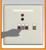
The Salvo SGL is placed over the emergency airline coupling releasing the trapped Salvo key and locking the Salvo SGL on. The trailer brakes are locked on. The Salvo key is then taken back to the Salvo Control Panel (SCP) at the loading bay.
