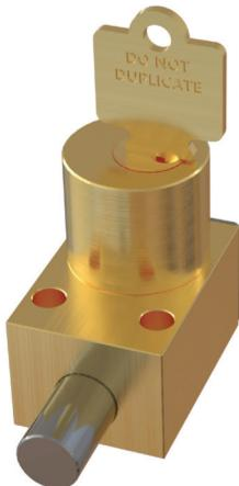
KIRK Type FF is the smallest of the KIRK bolt interlocks. It is a key operated mechanical interlock that is suitable for electrical switchgear. The standard unit comes with a stainless steel 1/2" diameter locking bolt with a throw or travel of 3/4". The locking bolt is used to inhibit or block the rotation or movement of operating handles or toggles of electrical switchgear. Many suppliers of switchgear equipment have mounting provisions available for KIRK interlocks.
