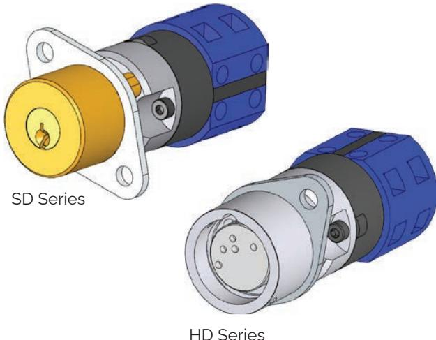
The KIRK Type PPS Power Panel Switch is a key actuated, rotary, two-position switch designed for isolation or switching of control circuitry. The Type PPS can be panel mounted or surface mounted with optional enclosure. It is available in switch ratings of 20, 25, 40, or 63A. The switch is UL listed and CSA approved.
