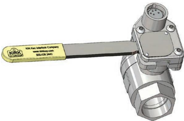
KIRK Type VL interlock is a key operated mechanical interlock that is suitable for the control and isolation of hazardous fluids or gases when performing maintenance on equipment. The standard unit comes pre-installed on a stainless steel  $\frac{1}{4}$ -turn ball valve and is ready for on-site installation. The lock is manufactured of stainless steel and the operation of the valve is lever controlled.
