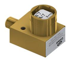
The K Lock is a key operated mechanical bolt interlock that is suitable for the control of electrical switchgear. The standard unit comes with a 15.88 mm diameter bolt available in various lengths, that is used to control the rotation or movement of operating handles or toggles of electrical switchgear. Many suppliers of switchgear equipment have mounting kits available for Castell interlocks. The lock is manufactured in brass or stainless steel.
