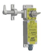
The AIS is a single key access interlock complete with electrical contacts for use on hinged doors. The AIS contacts can be used to switch off the machine via its control circuitry or to initialize a signal to visual beacons/sounders. The switch is sealed to IP65 with, 1 N/O 2 N/C contacts, rated to 10 A making it ideal for use in cross monitored safety systems. The interlock is manufactured in a durable stainless steel.
