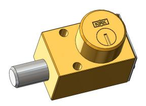
KIRK Type NT interlock is a key operated mechanical interlock that is suitable for the control of electrical switchgear. The standard unit comes with a stainless steel 5/8" diameter locking bolt with a throw or travel of 3/4". The locking bolt is used to control the rotation or movement of operating handles or toggles of electrical switchgear. Many suppliers of switchgear equipment have mounting provisions available for KIRK interlocks.
