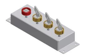
The X key exchange box is designed to enable the release of keys by the insertion of one or more free key(s). The need for this type of product usually arises when there are multiple points of entry. The unit will generally be the link between the isolation locks and the access products. The product is supplied in a housing suitable for surface mounting and is available in a number of configurations and number of locks.
